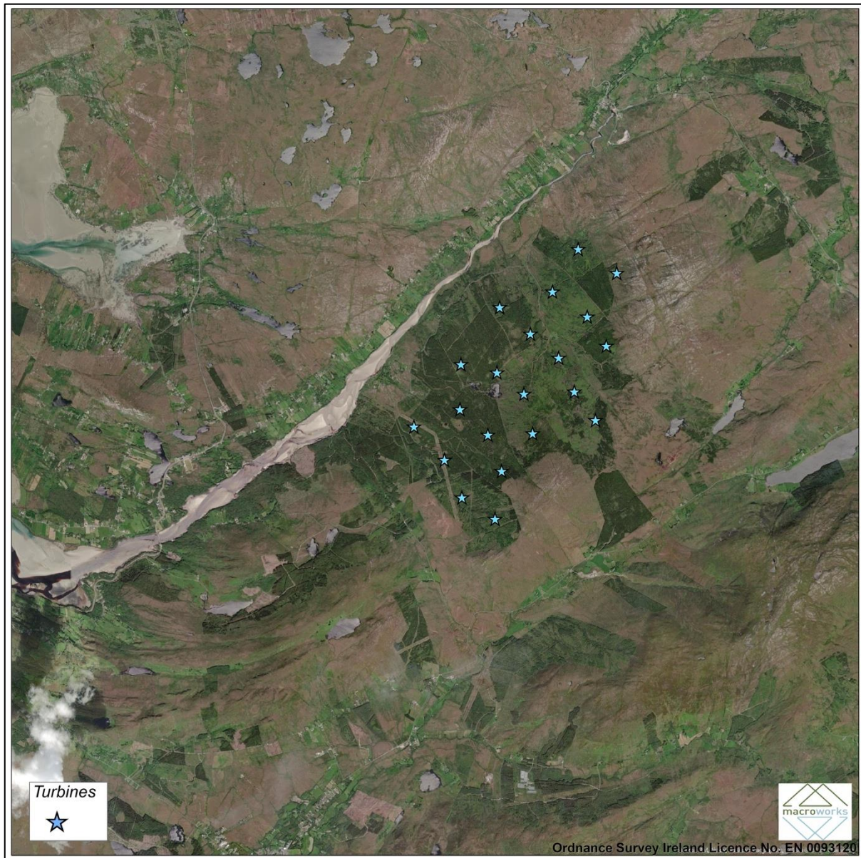
Figure 13-13: DI2 layout comprising 21 turbines
